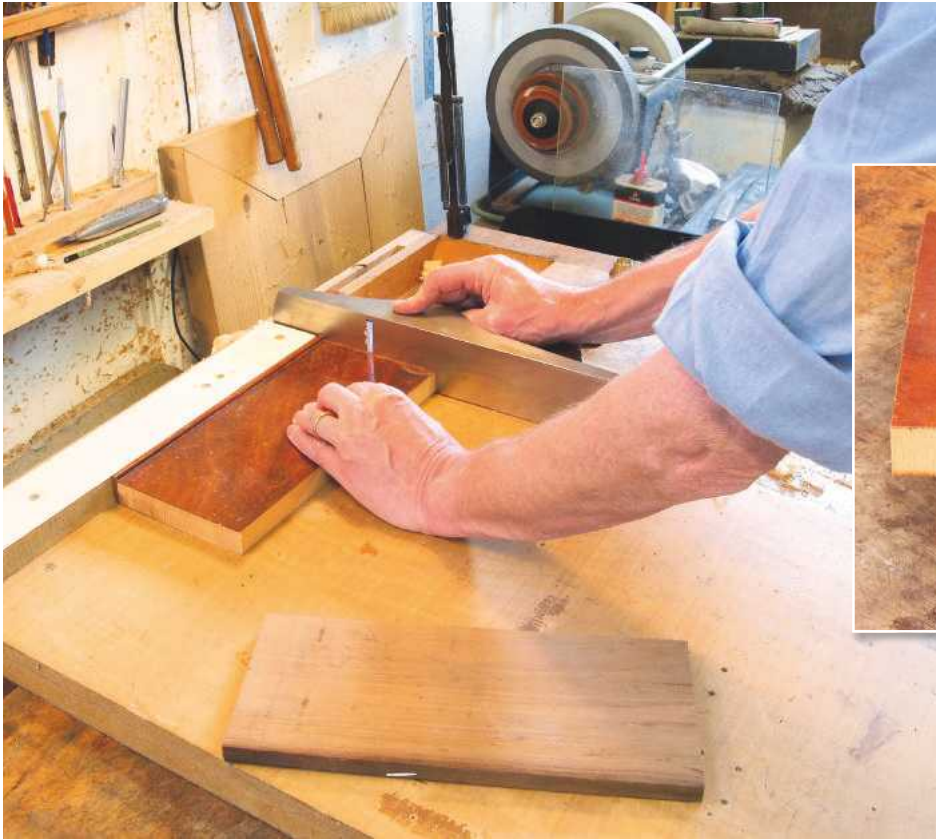
▲ Pic.1 Planing edges square on shooting board and, inset, showing bowed timber
